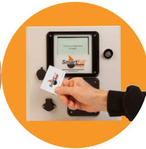
Once authorised, the unit can request the vehicle speed/hourmeter reading and/or job number, which helps with scheduling maintenance
