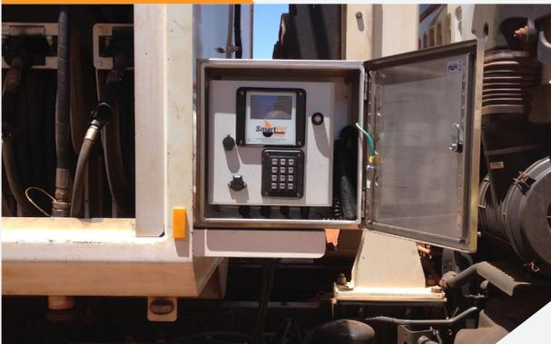
With auto power off and battery isolation, the system has been specifically designed for service truck use.
