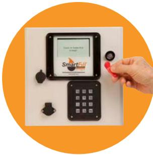
Touch the authorised vehicle ID key, fob or NFC card onto the sensor of the unit
